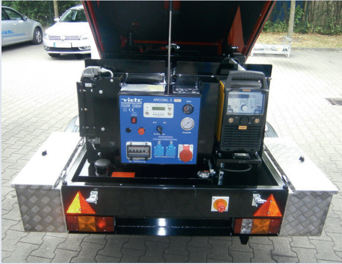
Welding inverter and subjacent associated insulating transformer
